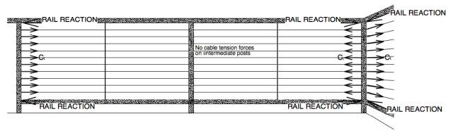
Cable tension forces occur where cables either change direction at the post or are terminated at a post. Top rail acts as a compression element to resist cable tension forces. The top rail infill piece inserts tight between the posts so that the post reaction occurs by direct bearing.
