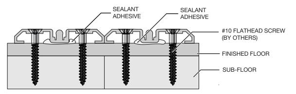
**Floor Structure-** The Finished Floor Surface and the supporting Sub-floor must be capable of supporting the BRS Sliding Door System. The design of the BRS100 system concentrates the load at the bottom track and not the head channel. Large, heavy glass panels may load the floor structure with several hundred pounds. Verify the load capacity of the floor with a Structural Engineer before installation.
