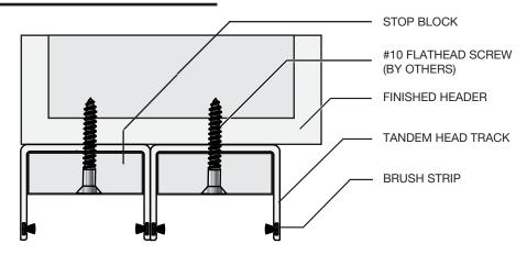
**Lateral Loading -** The BRS Head Track must be mounted to a structurally sound finished Opening Header capable of supporting repeated lateral loads during operation. Verify the load capacity with a Structural Engineer before installation.
