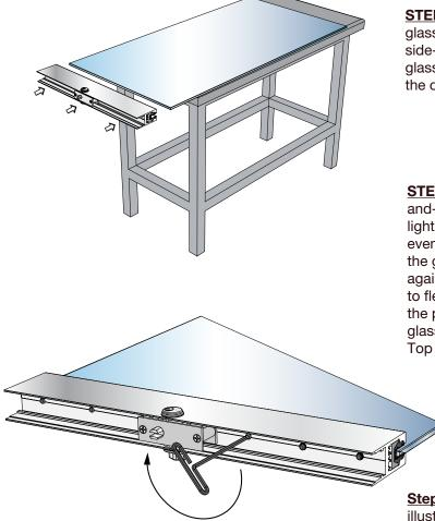
**STEP 1:** Slide the Bottom HERC Rail over the end of the glass panel and snug against the edge. Center the rail side-to-side. **NOTE:** If the HERC Rail will not fit over the glass, loosen the set screws along the bottom to spread the clamp rails.
