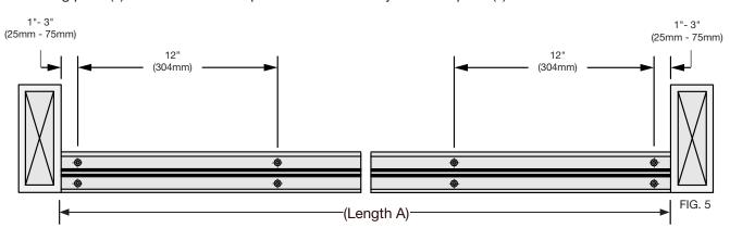
STEP 1: Measure and cut track profiles to fit between finished walls or jambs. (Length A)
