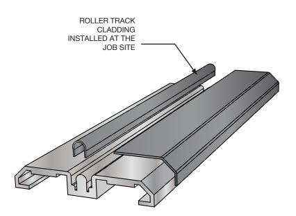
**IMPORTANT:** Bottom track cladding should be applied before installing rolling and fixed panels.
