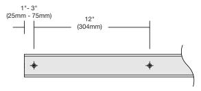
**STEP 2:** Mount the sections of the Fixed Track to the finished floor surface using #10 X 2" or equivalent fasteners while maintaining a 1/8" (3mm) gap between the two tracks.
