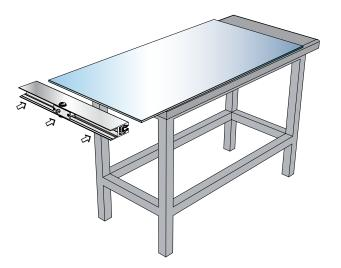
**STEP 1**: Slide the bottom HERC-DOOR® Rail over the end of the glass panel and snug against the edge. Center the rail side-to-side. NOTE: If the HERC-DOOR® Rail will not fit over the glass, loosen the set screws along the bottom to spread the clamp rails.
