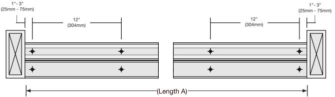
STEP 1: Measure and cut track profiles to fit between finished walls or jambs. (Length A)
