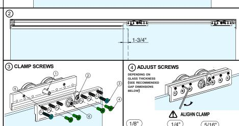
(1) HEIGHT ADJUSTMENT SCREW (2) ANTIJUMP SCREW (3) CLAMP TIGHTEN SCREW: (x2) GLASS 3/8" -- (x6) GLASS 1/2" -- (x6) GLASS 9/16")
