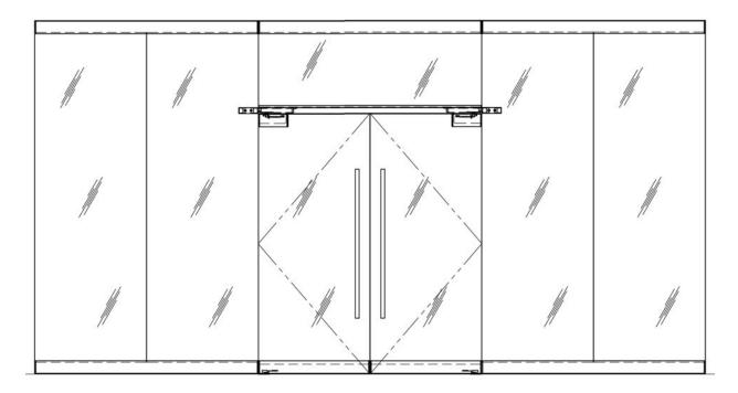
The header supports wind load reactions from the door hinges as well as dead load and wind load reactions from the transom. The ends of the header are attached to the side lites which carry the reactions to the structure. The side lites must be checked for the point load condition.
