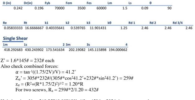
Hole bearing,  $V_a = 2*0.25"*0.09"*30$ ksi/3 = 450# > 232# does not control Pullover,  $T_a = (0.5"-0.25")*0.09"*25$ ksi/3 = 188# < 305# controls
