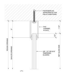
uniform reaction = w w = hP/2 (Where h<sub>t</sub> is the height of the transom or sidelite and P is the wind pressure) V = w\*1' T = w\*1'\*2"/0.5" = 4w T<sub>a</sub> < 4V<sub>a</sub> so tension loading on fastener controls w<sub>a</sub> = 301#/4 = 75.3plf P<sub>a</sub> = 75.3plf\*2/h
