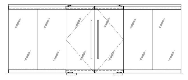
Door hinges attach directly to the structure and the side lites are unaffected by loading on the door.
