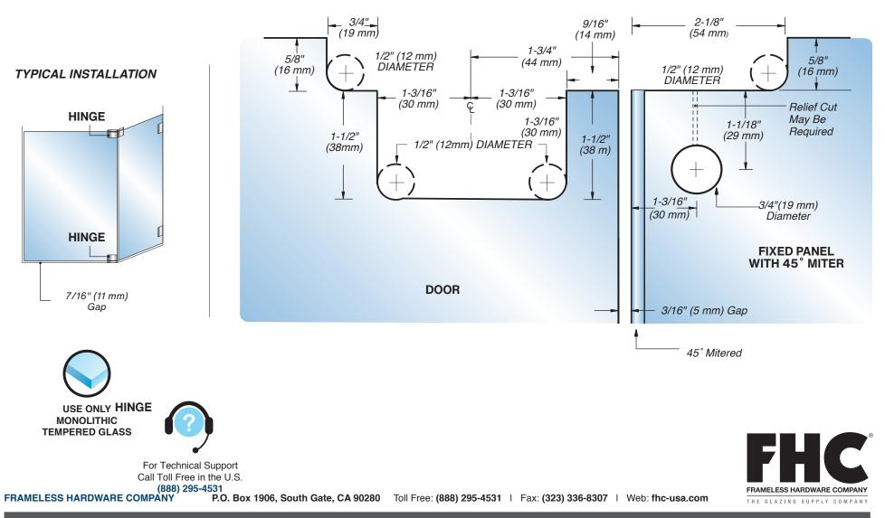
135° Glass-to-Glass Hinge With Attached U-Clamp ITEM NO. PAT0735L (Left Hinge) ITEM NO. PAT0735R (Right Hinge)
