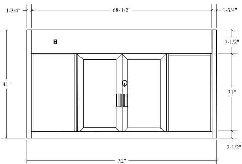
ALL QUIKSERV PRODUCTS ARE SHIPPED FULLY-ASSEMBLED and READY TO INSTALL. EACH ELECTRICAL UNIT IS SHIPPED WITH A FOUR FOOT (4') BX DROP.
