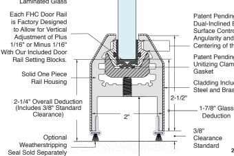
Patent Pending **Dual-Inclined Bearing** Surface Controls Angularity and Self Centering of the Rail
