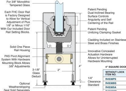
Patent Pending **Dual-Inclined Bearing** Surface Controls Angularity and Self Centering of the Rail
