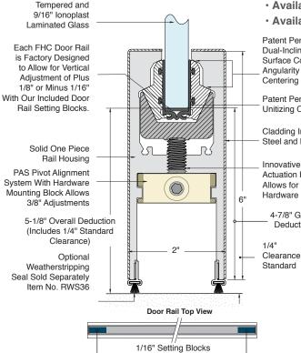
**Dual-Inclined Bearing** Surface Controls Angularity and Self Centering of the Rail
