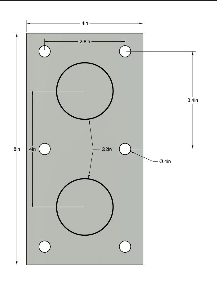
tested for  $\frac{11}{16}$ " and  $\frac{13}{16}$ " laminated glass consult an engineer if using  $\frac{9}{16}$ " laminated glass type 316 SS  $\emptyset^{3}_{4}$ " glass hole
