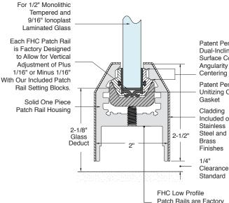
Patent Pending **Dual-Inclined Bearing** Surface Controls Angularity and Self Centering of the Patch Rail
