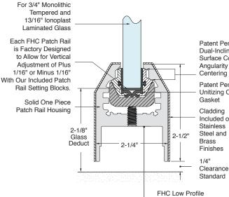
Patent Pending **Dual-Inclined Bearing** Surface Controls Angularity and Self Centering of the Patch Rail
