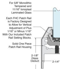
Patent Pending Dual-Inclined Bearing Surface Controls Angularity and Self Centering of the Patch Rail Patent Pending Unitizing Clamping
