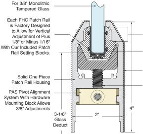
Patent Pending **Dual-Inclined Bearing** Surface Controls Angularity and Self Centering of the Patch Rail
